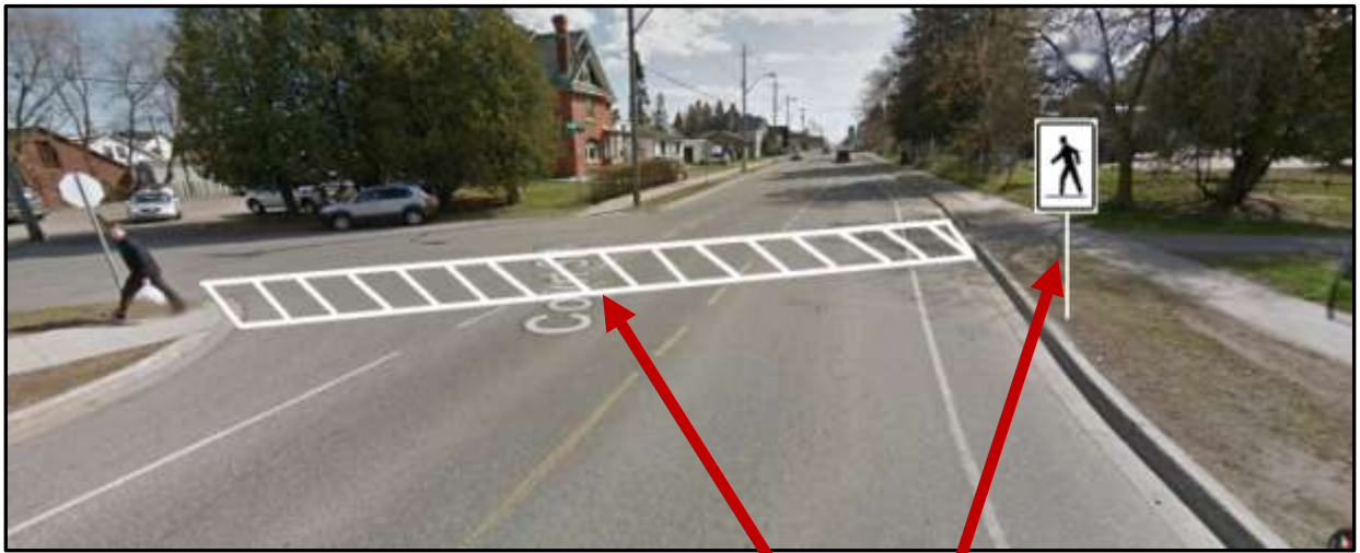
Pedestrian crossing of Court Street needs proper pavement markings, lighting, and signage to alert drivers for improved pedestrian safety
